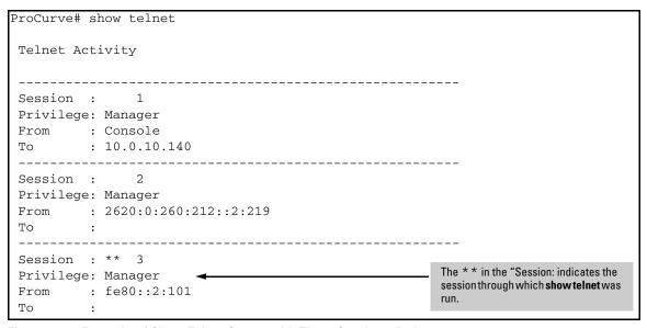
Figure 5-4. Example of Show Telnet Output with Three Sessions Active
